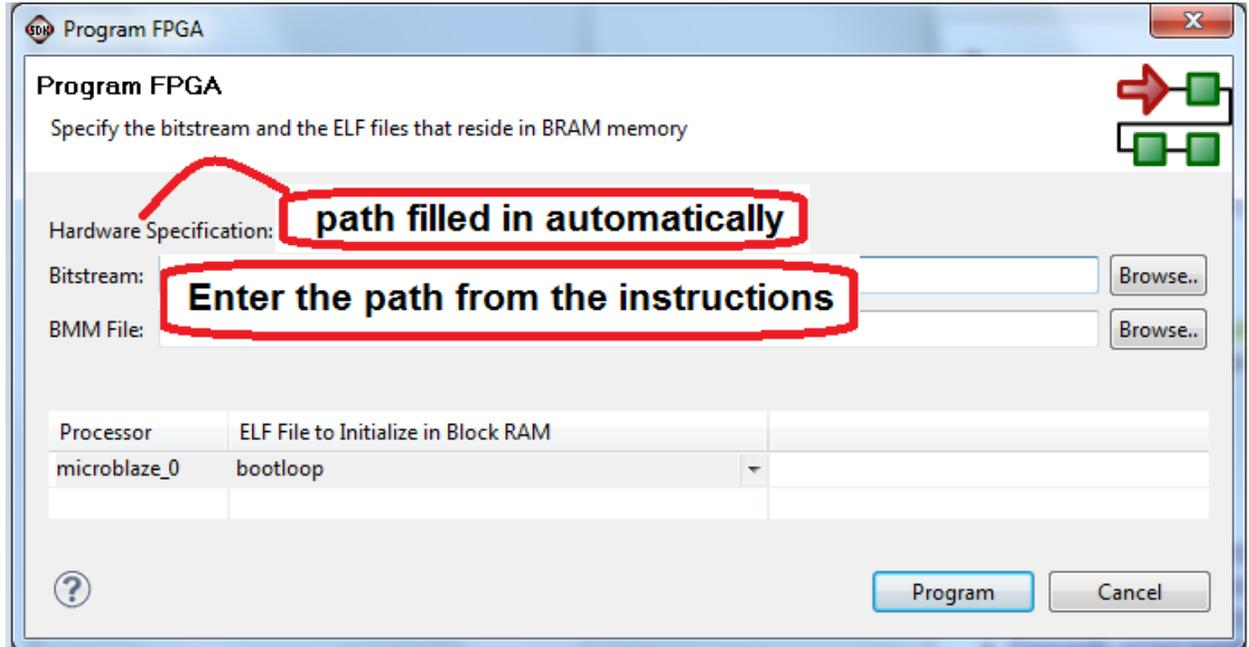
It takes approximately 10 seconds to download the FPGA and a message box indicating **FPGA configuration complete** appears.
