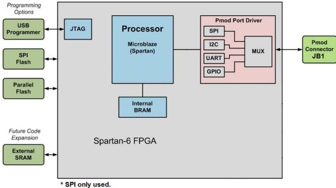
**Figure 3. Block Diagram of FPGA Hardware Design**
