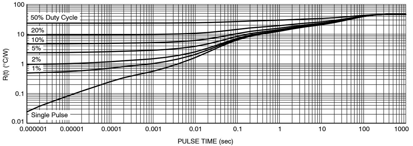
Figure 13. Thermal Characteristics
