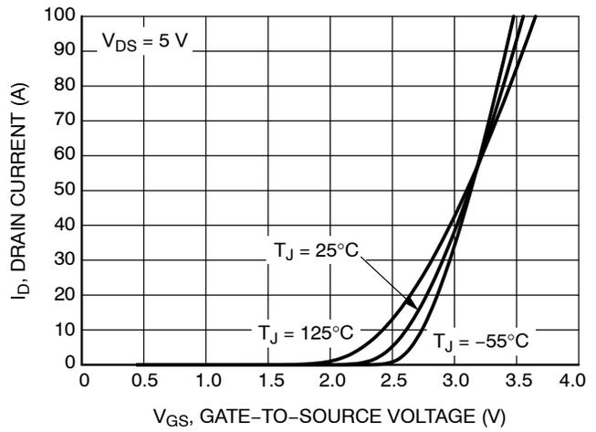
Figure 2. Transfer Characteristics
