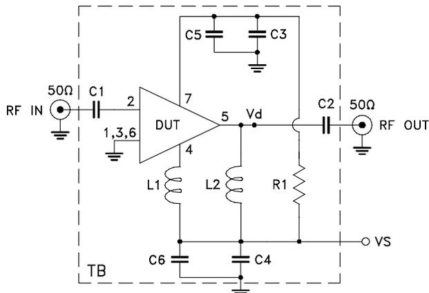
**Fig 1.** Block Diagram of Test Circuit used for characterization. (DUT soldered on Mini-Circuits Characterization Test Board TB-607+-2) Gain, Output power at 1dB compression (P1dB), Output IP3 (OIP3), Noise Figure are measured using Agilent’s N5242A PNA-X microwave network analyzer.
