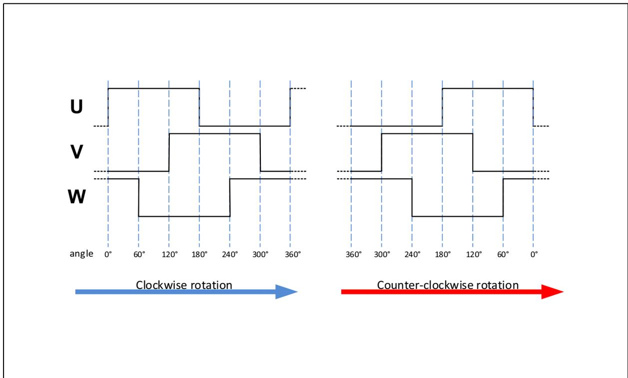
The [Figure 33](#) shows the UVW signal flow if the magnet rotates in clockwise direction and counter-clockwise direction (DIR=0). In case of clockwise rotation when the magnet is rotating to the right hand side, the angle value is increasing. Clockwise rotation direction is defined as shown in [Figure 44](#). With the bit DIR, it is possible to invert the rotation direction.
