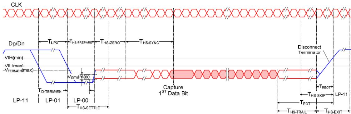
Figure 13.2: Timing of high-speed data transmission in bursts
