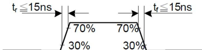
8.1.5 Parallel 18/16/6-bit RGB Interface Timing Characteristics
