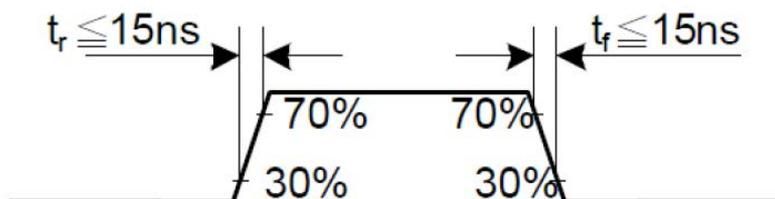
8.1.4 Display Serial Interface Timing Characteristics (4-line SPI system)
