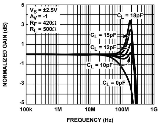
FIGURE 13. INVERTING FREQUENCY RESPONSE FOR VARIOUS  $C_L$
