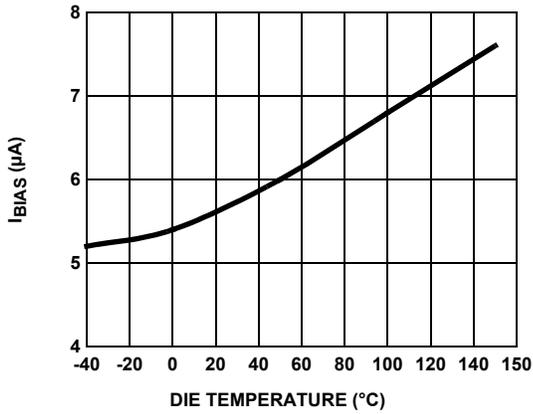
FIGURE 41.  $I_{BIAS}$  CURRENT vs TEMPERATURE
