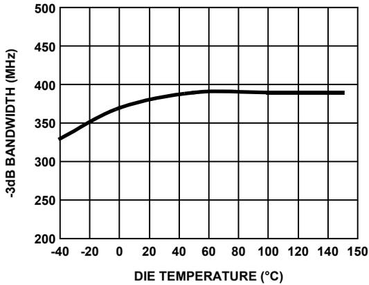
FIGURE 37. -3dB BANDWIDTH vs TEMPERATURE
