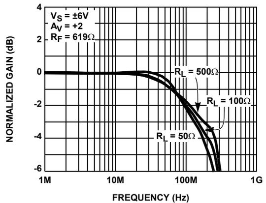
FIGURE 4. NON-INVERTING FREQUENCY RESPONSE FOR VARIOUS  $R_L$
