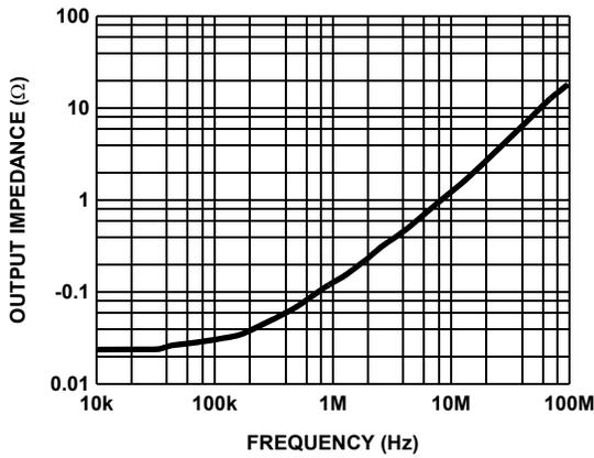
FIGURE 29. CLOSED LOOP OUTPUT IMPEDANCE vs FREQUENCY
