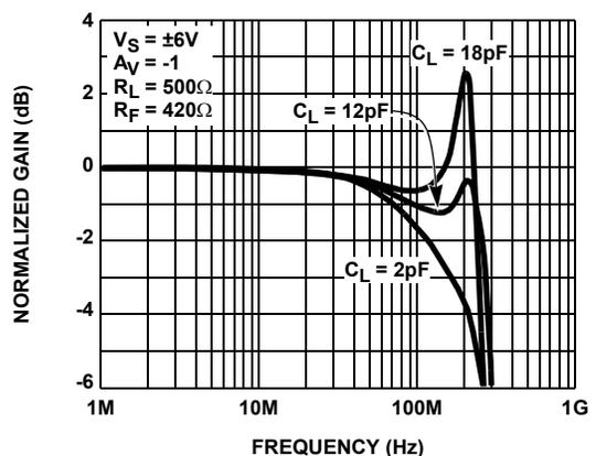
FIGURE 8. INVERTING FREQUENCY RESPONSE FOR VARIOUS  $C_L$
