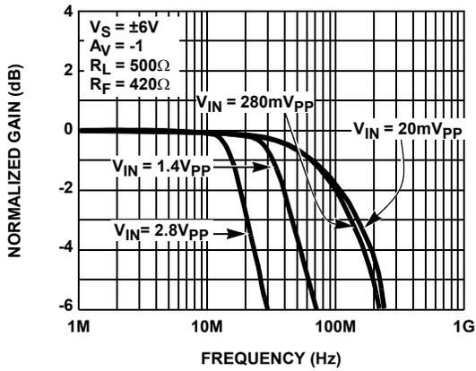
FIGURE 9. INVERTING FREQUENCY RESPONSE FOR VARIOUS SIGNAL LEVELS
