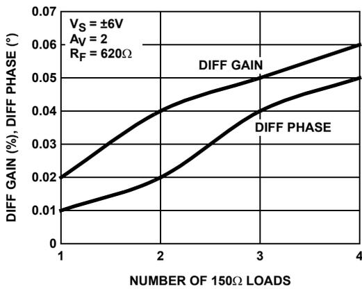
FIGURE 31. DIFFERENTIAL GAIN/PHASE
