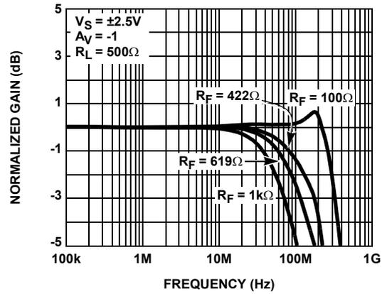
FIGURE 10. INVERTING FREQUENCY RESPONSE FOR VARIOUS  $R_F$
