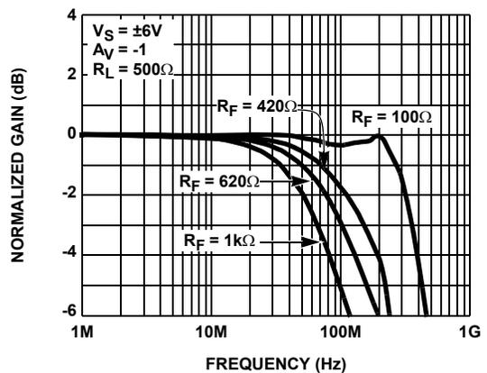
FIGURE 6. INVERTING FREQUENCY RESPONSE FOR VARIOUS  $R_F$
