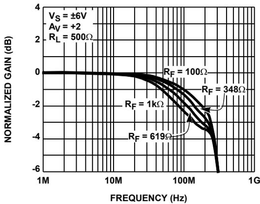
FIGURE 1. NON-INVERTING FREQUENCY RESPONSE FOR VARIOUS  $R_F$
