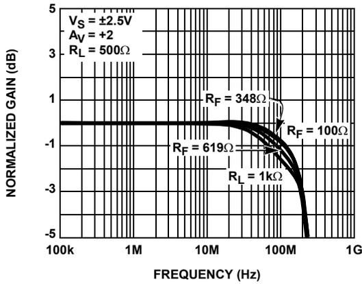
FIGURE 15. NON-INVERTING FREQUENCY RESPONSE FOR VARIOUS  $R_F$
