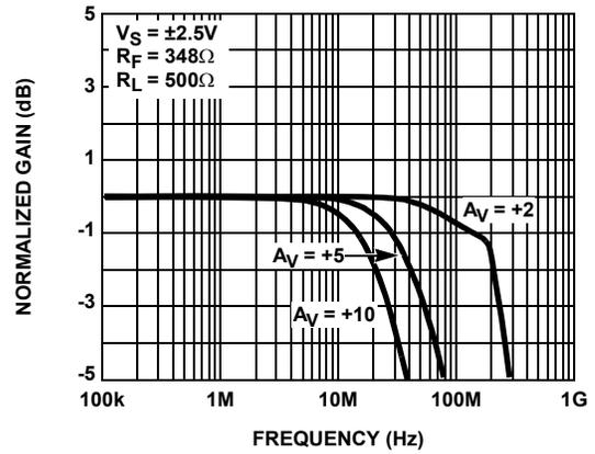
FIGURE 16. NON-INVERTING FREQUENCY RESPONSE FOR VARIOUS  $A_V$
