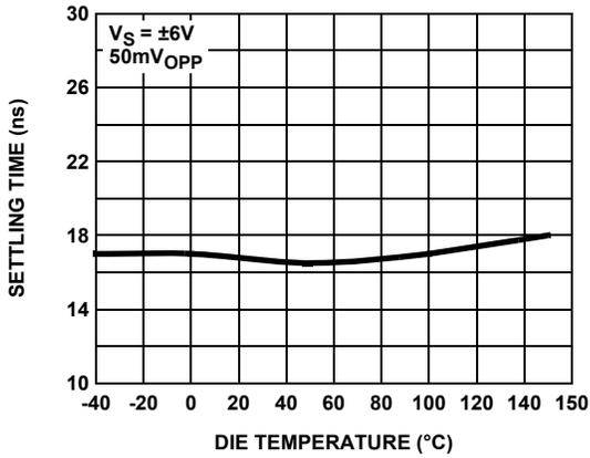
FIGURE 39. 0.1% SETTILING TIME vs TEMPERATURE
