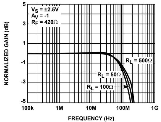
FIGURE 12. INVERTING FREQUENCY RESPONSE FOR VARIOUS  $R_L$
