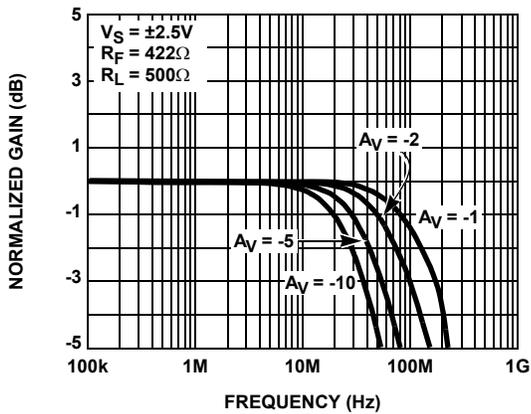
FIGURE 11. INVERTING FREQUENCY RESPONSE FOR VARIOUS  $A_V$
