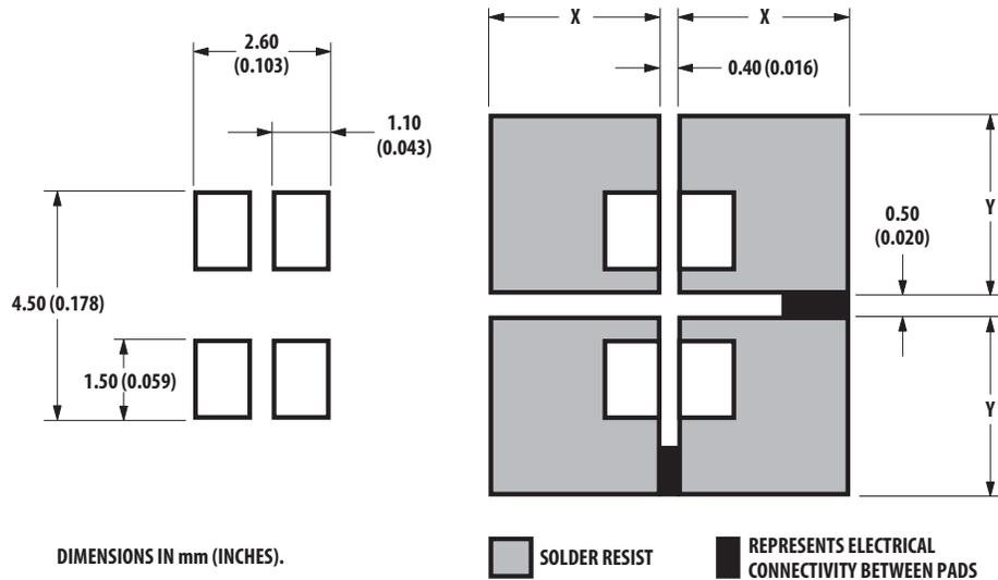
Figure 8a. Recommended soldering pad pattern
