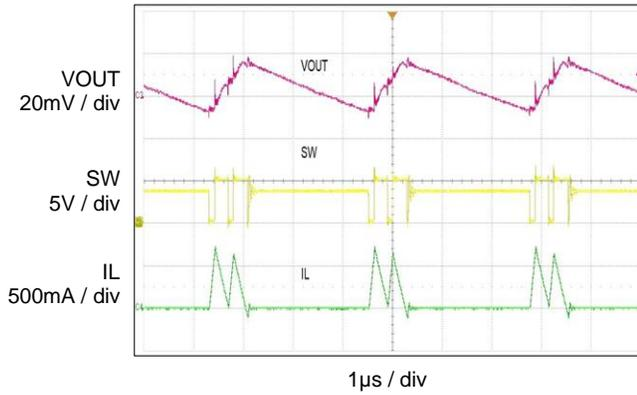
**Switching waveform 350mA load (PWM mode)**
