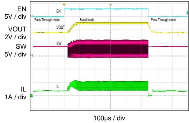
**Switching waveform 50mA load (PFM mode)**
