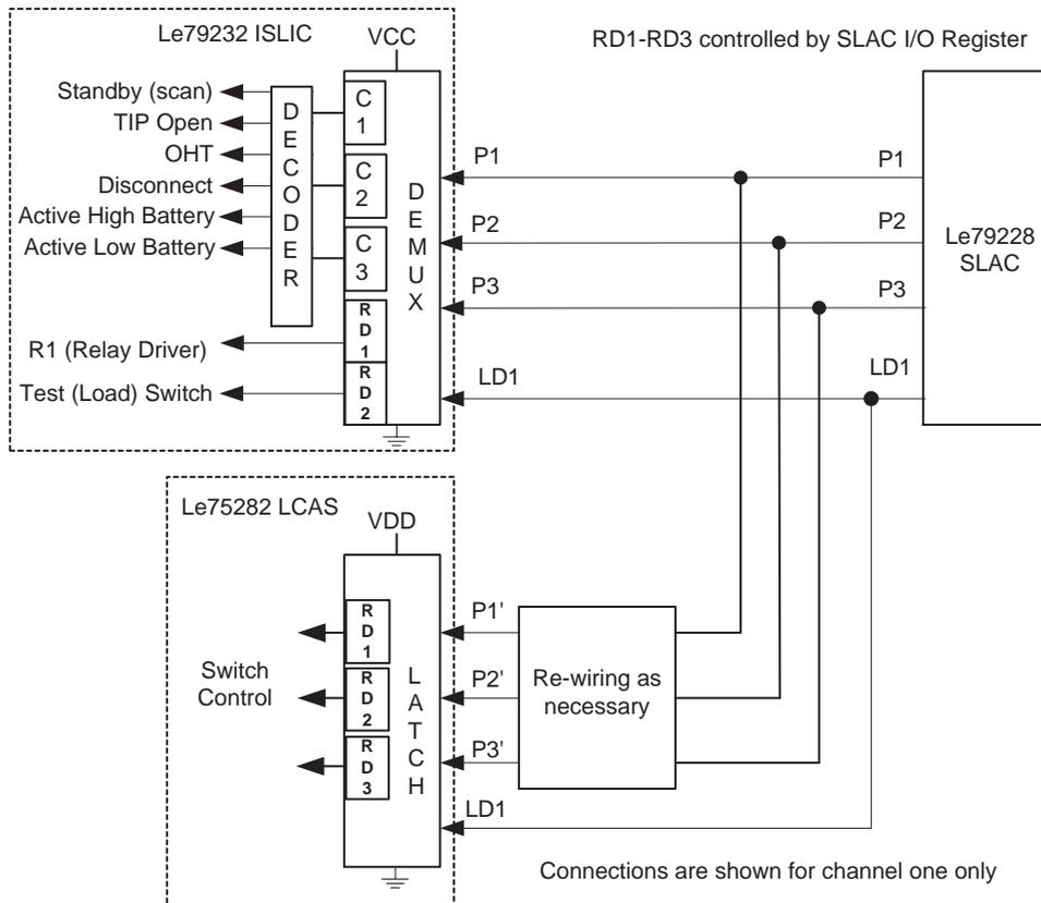
Control and wiring scenarios for the ISLIC device and LCAS device follows.
