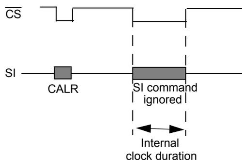
In case of negative  $\overline{CS}$  pulse is outside a predefined time range (from  $t_{CSB(MIN)}$  to  $t_{CSB(MAX)}$ ), the calibration event will be ignored and the internal clock will be unaltered or reset to default value ( $f_{PWM(0)}$ ) if this was not calibrated before.
