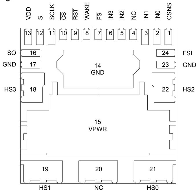
Figure 3. 10XS3412 Pin Connections
