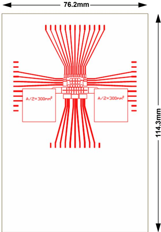
Figure 16. 1s JEDEC Thermal Test Board Layout
