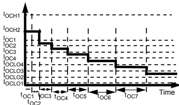
**Figure 14. Overcurrent profile with OCHI bit set to '1'**
