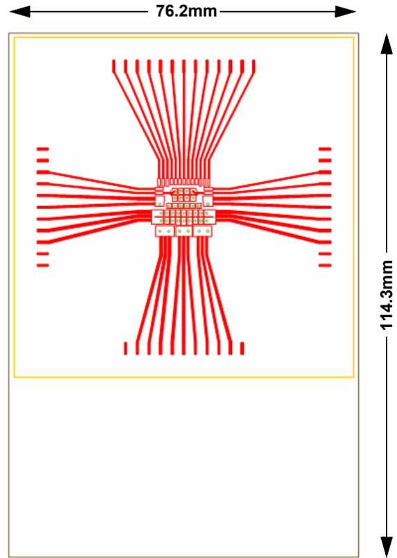
Figure 17. 2s2p JEDEC Thermal Test Board
