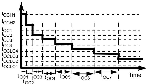
**Figure 13. Overcurrent profile depending on Xenon bit**
