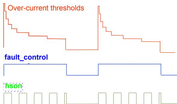
In steady state, the wire harness will be protected by OCLO2 current level by default. Three other DC overcurrent
