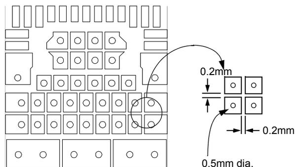
Figure 15. Detail of Copper Traces Under Device with Thermal Vias
