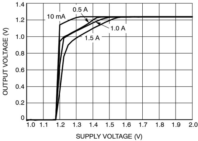
**Figure 6. Dropout Characteristics**
