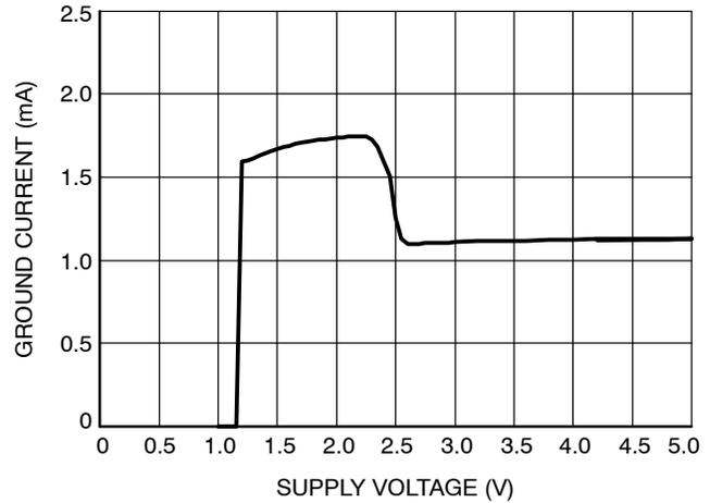
**Figure 11. Ground Current vs. Supply Voltage**
