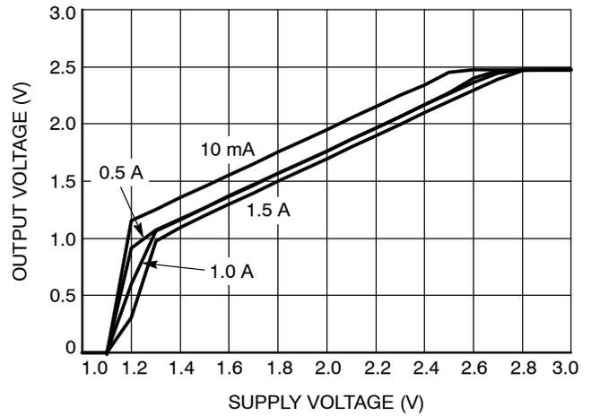
**Figure 7. Dropout Characteristics**
