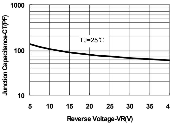
Fig.1-Typical Junction Capacitance
