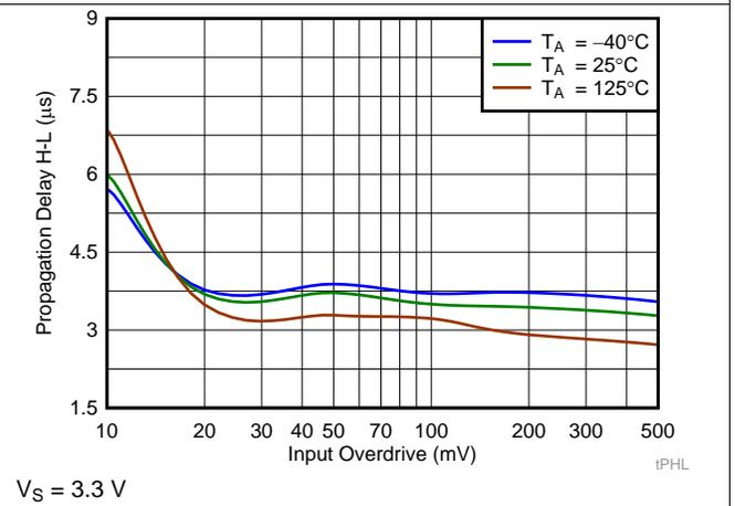
Figure 6. Propagation Delay (H-L) vs. Input Overdrive
