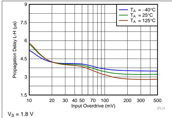
Figure 3. Propagation Delay (L-H) vs. Input Overdrive
