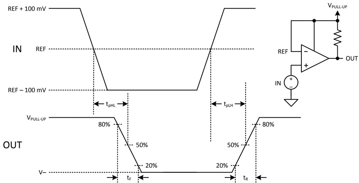
Figure 2. Timing Diagram
