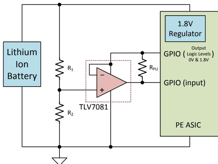
Figure 23. Battery Monitor
