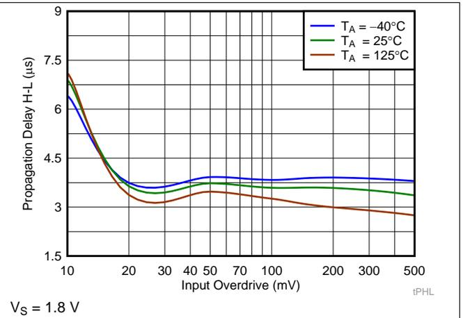
Figure 4. Propagation Delay (H-L) vs. Input Overdrive
