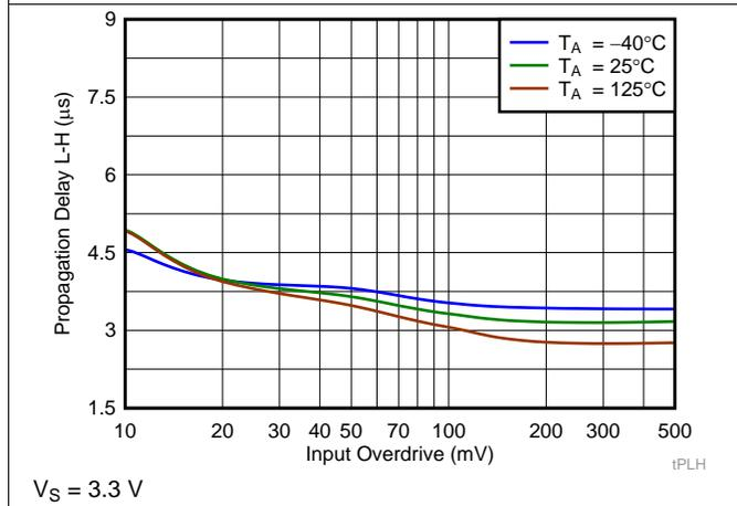
Figure 5. Propagation Delay (L-H) vs. Input Overdrive
