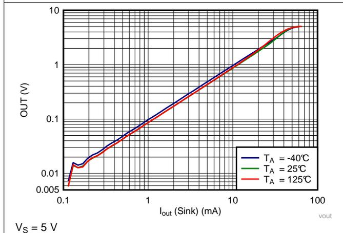
Figure 11. Output Voltage Low vs. Output Sink Current
