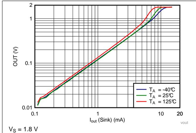
Figure 9. Output Voltage Low vs. Output Sink Current
