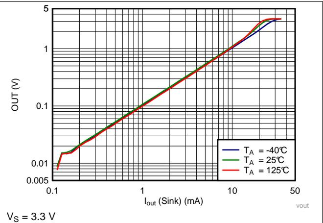
Figure 10. Output Voltage Low vs. Output Sink Current
