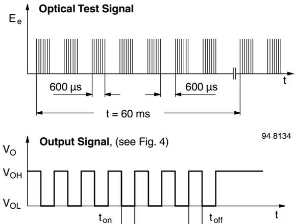
Fig. 3 - Test Signal
