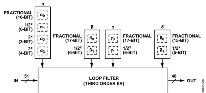
Figure 42. Third Order Digital IIR Loop Filter
