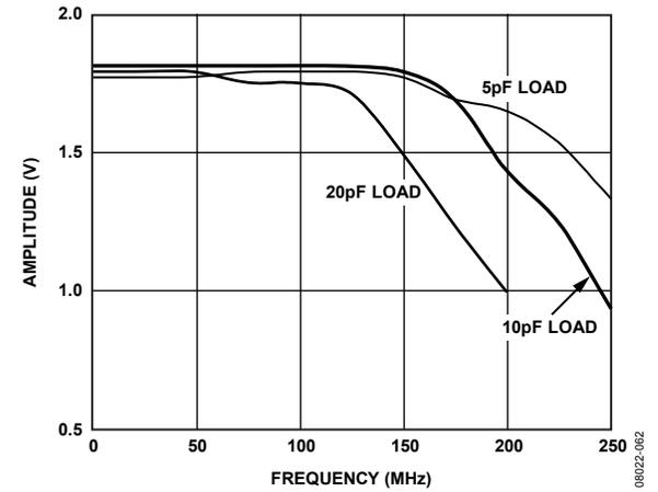
Figure 17. Amplitude vs. Toggle Rate, 1.8 V CMOS
