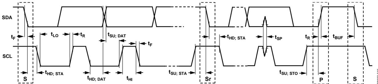
Figure 67. I<sup>2</sup>C Serial Port Timing
