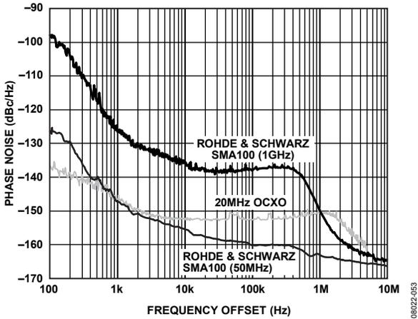
Figure 13. Phase Noise of SYSCLK Input Sources
