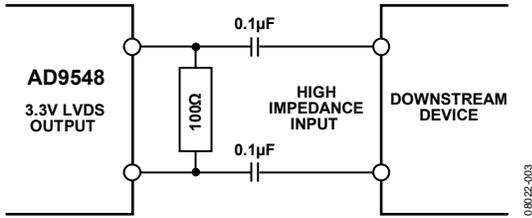
Figure 28. AC-Coupled LVDS or LVPECL Output Driver
