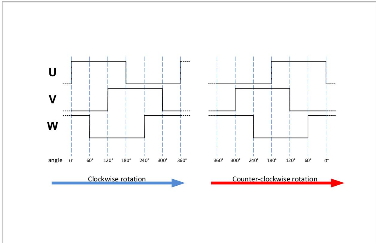
The Figure 54 shows the UVW signal flow if the magnet rotates in clockwise direction and counter-clockwise direction (DIR=0). The rotation direction of the magnet is defined as clockwise (DIR=0) when the view is from the topside of AS5x47U. With the bit DIR, it is possible to invert the rotation direction.
