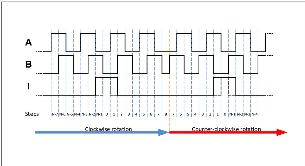
N = 16384 for 14-bit resolution, N = 4096 for 12-bit resolution and N = 1024 for 10-bit resolution..
