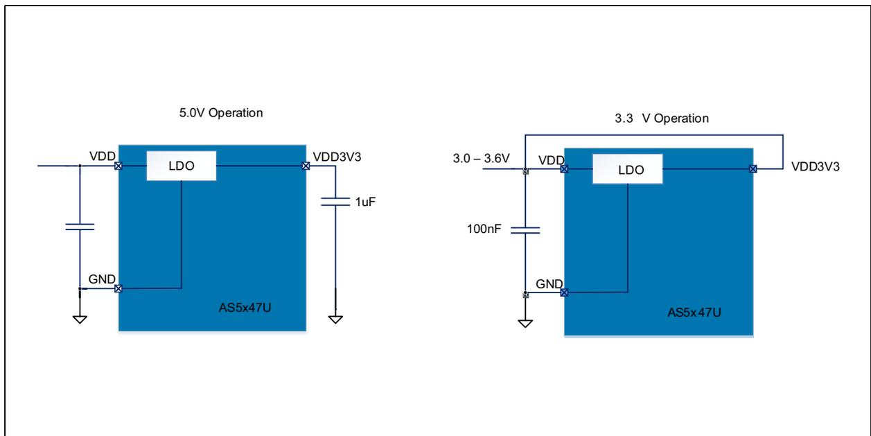
Setting valid for one sensor IC. Double setting necessary for AS5247U.
