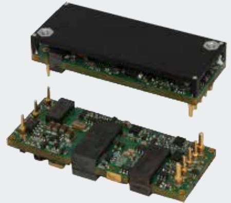
Advanced Energy's Artesyn AVO120 series eighth-brick isolated DC-DC converter is designed specifically to provide a regulated low noise 12 Vdc output for feeding downstream non-isolated point-of-load (POL) converters in systems with distributed power architectures (DPA). Rated at 120 watts, it can deliver up to 10 amps. The converter has a wide 2:1 input range of 36 to 75 Vdc and is designed primarily for use with standard 48 V telecommunications equipment supplies.
