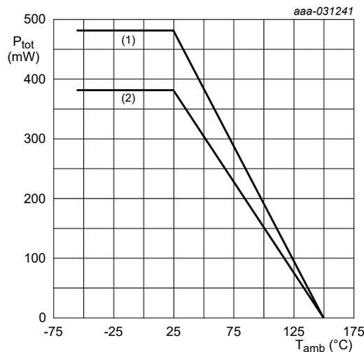
(1) FR4 PCB; single-sided 70  $\mu\text{m}$  copper, tin-plated and standard footprint
