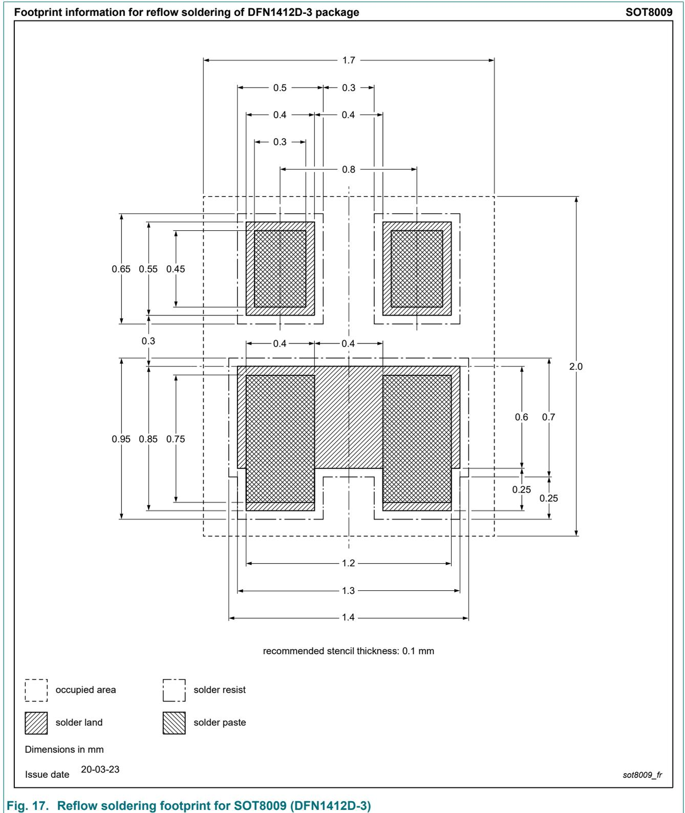
**Fig. 17. Reflow soldering footprint for SOT8009 (DFN1412D-3)**
