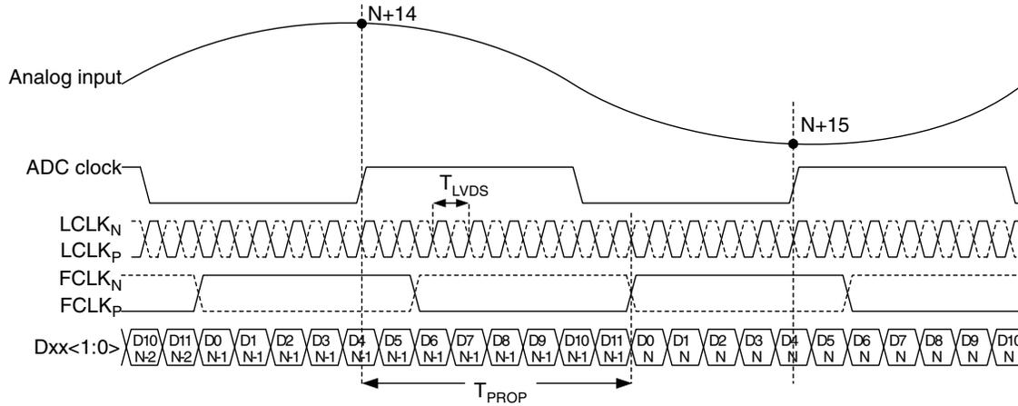
Figure 6. LVDS timing 12 bit output, SDR mode
