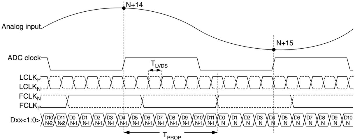
Figure 4. LVDS timing 12 bit output, DDR mode
