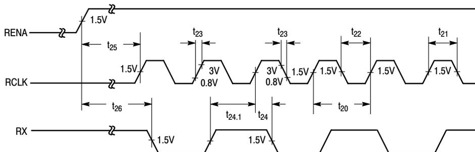
Figure 12. Receive Timing (Motorola End of Frame)
