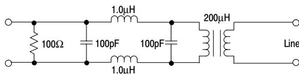
Figure 31. TPRX Input Switching
