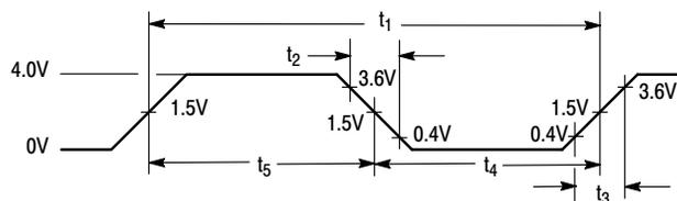
Figure 9. Receive Phase-Locked-Loop Switching
