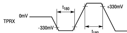
Figure 32. TPRX Receive Timing (Start of Frame)
