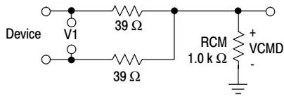
Figure 4. Test Load B2
