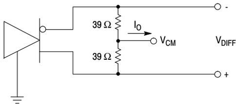
Figure 7. AUI Differential Output Short Circuit Current
