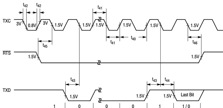
Figure 14. Receive Timing (Intel)
