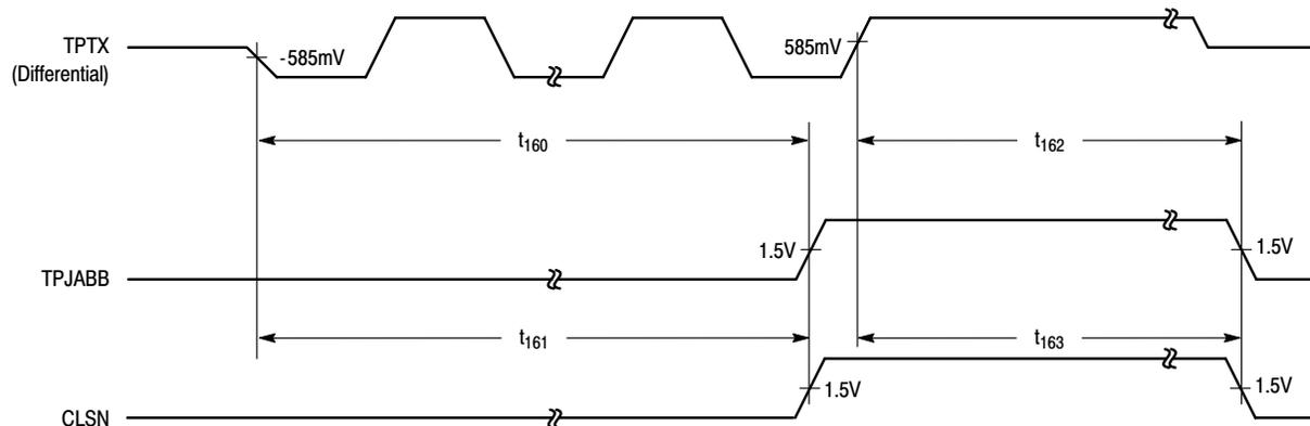
Figure 29. TPTX SQE (CLSN) Timing (End of Frame)
