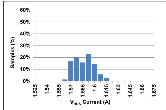
**FIGURE 2-17:** ILIM5 Trip Current Distribution<sup>(1)</sup>.
