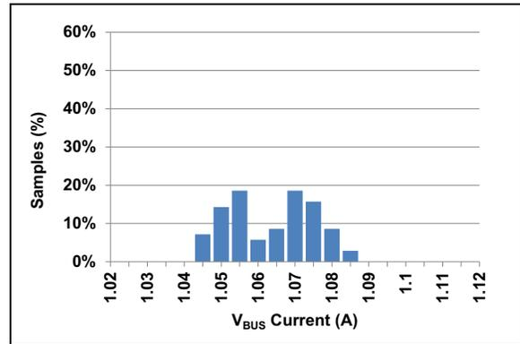
**FIGURE 2-15:** ILIM3 Trip Current Distribution<sup>(1)</sup>.
