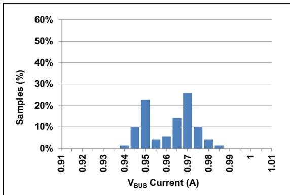
**FIGURE 2-14:** ILIM2 Trip Current Distribution<sup>(1)</sup>.
