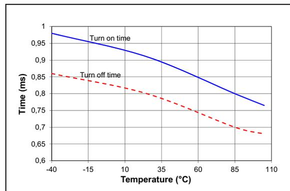
**FIGURE 2-6:** Power Switch On/Off Time vs. Temperature.
