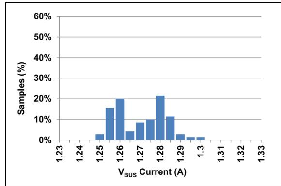
**FIGURE 2-16:** ILIM4 Trip Current Distribution<sup>(1)</sup>.
