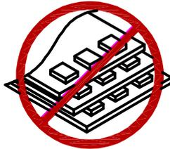
4. As silicone encapsulation is permeable to gases, some corrosive substances such as H<sub>2</sub>S might corrode silver plating of leadframe. Special care should be taken if an LED with silicone encapsulation is to be used near such substances.
