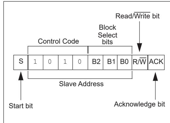
**FIGURE 5-2: ADDRESS SEQUENCE BIT ASSIGNMENTS**
