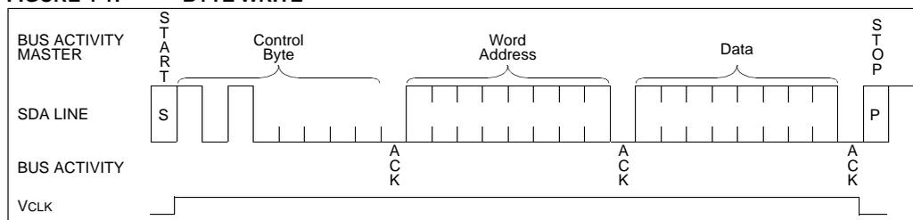
**FIGURE 4-2: BYTE WRITE**
