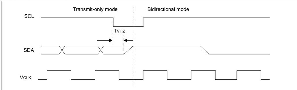
**FIGURE 3-2: DATA TRANSFER SEQUENCE ON THE SERIAL BUS**
