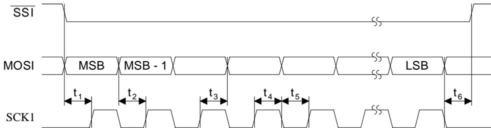
**Figure 4. MOSI Write Timing in SPI Slave Mode**
