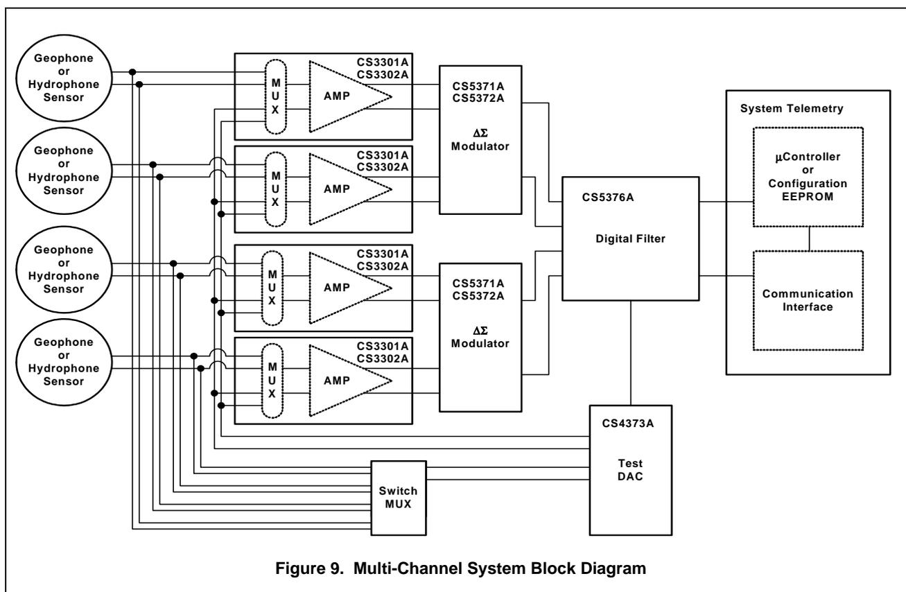
Figure 9. Multi-Channel System Block Diagram
