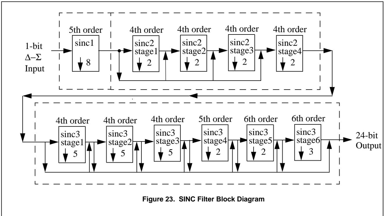
Figure 23. SINC Filter Block Diagram
