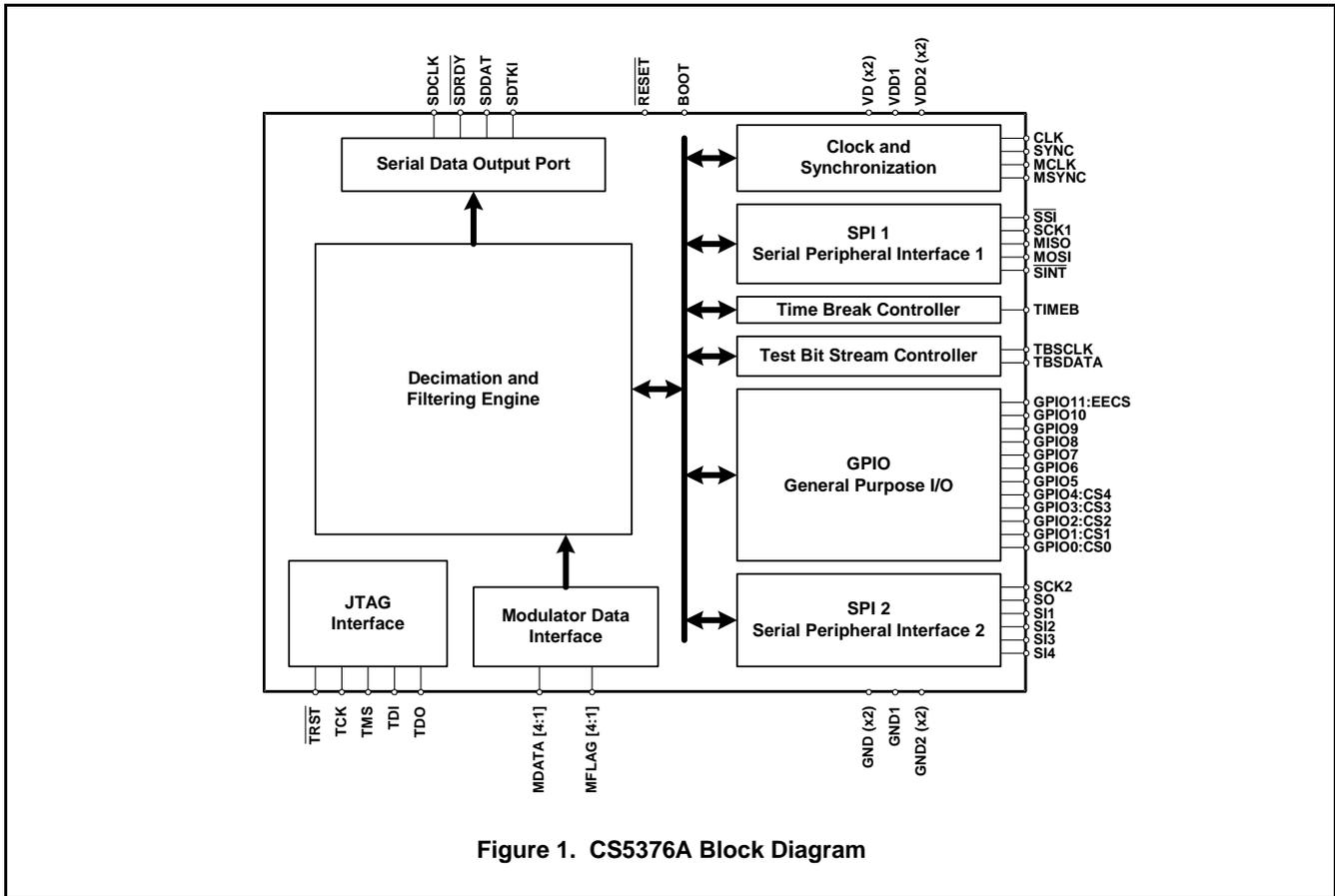
Figure 1. CS5376A Block Diagram
