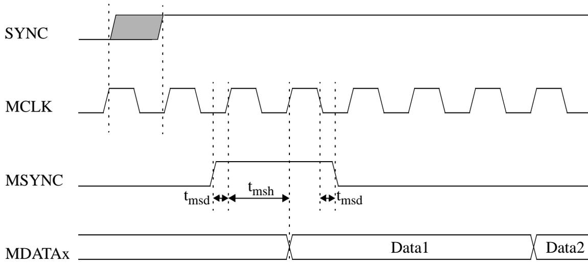
Note: SYNC input latched on MCLK rising edge. MSYNC output triggered by MCLK falling edge.
