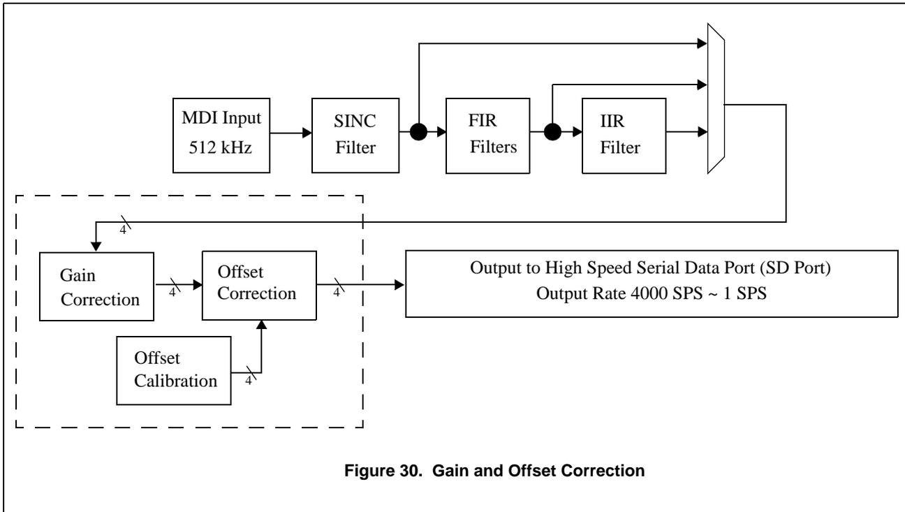
Figure 30. Gain and Offset Correction
