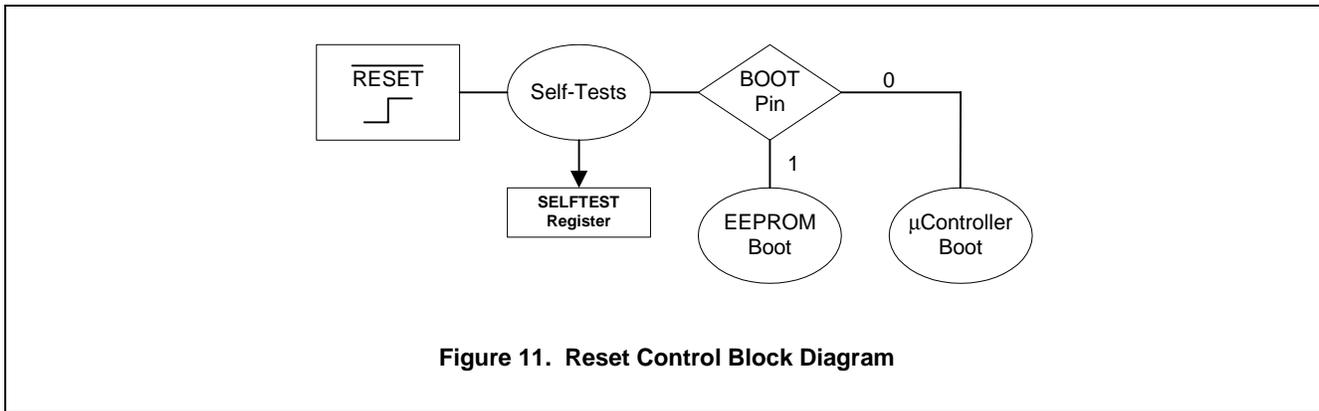
**Figure 11. Reset Control Block Diagram**
