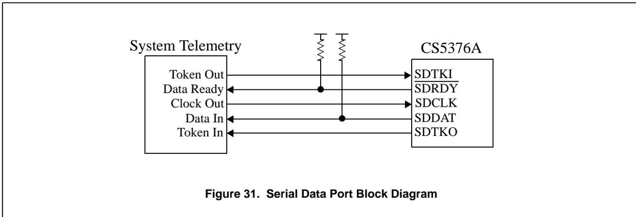
Figure 31. Serial Data Port Block Diagram
