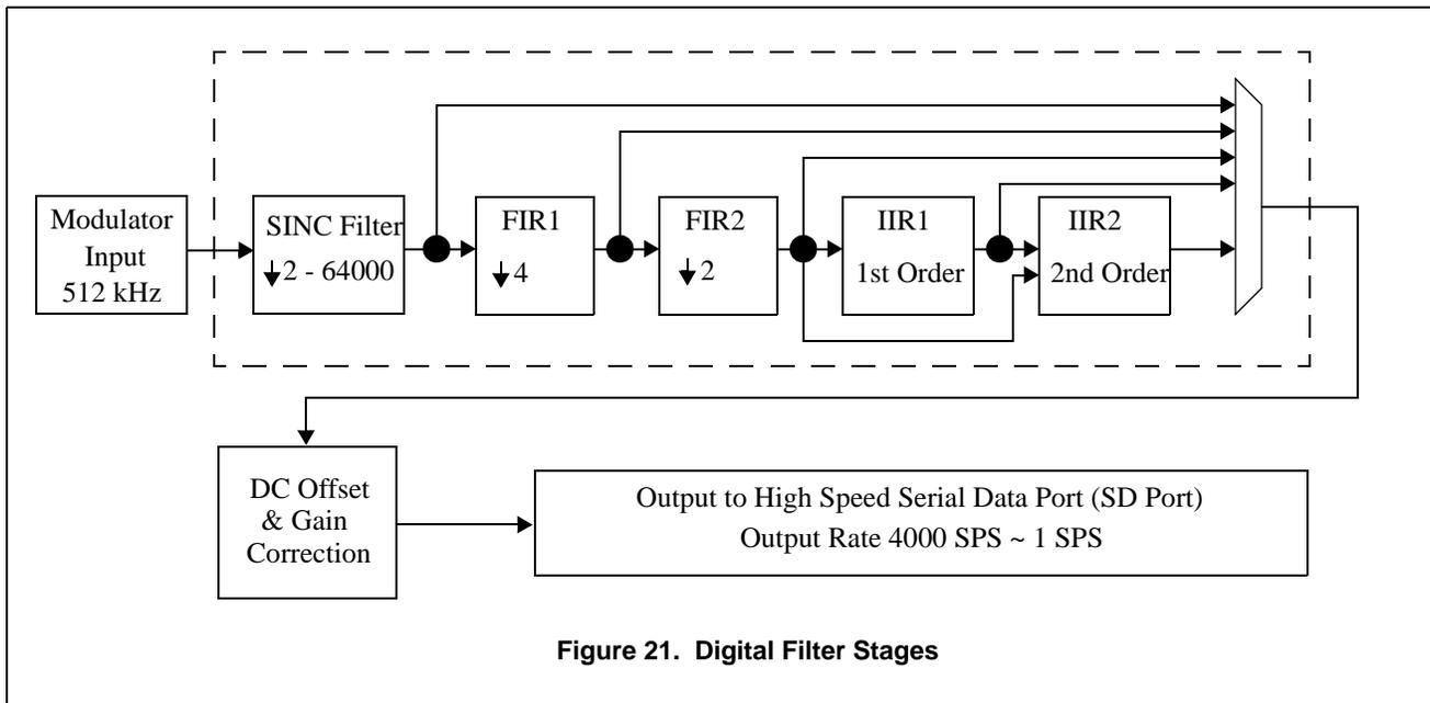
**Figure 21. Digital Filter Stages**
