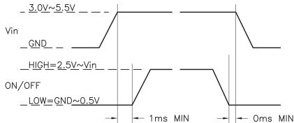
Until Vin voltage reaches the spec voltage, it does not change ON/OFF function from LOW to HIGH.
