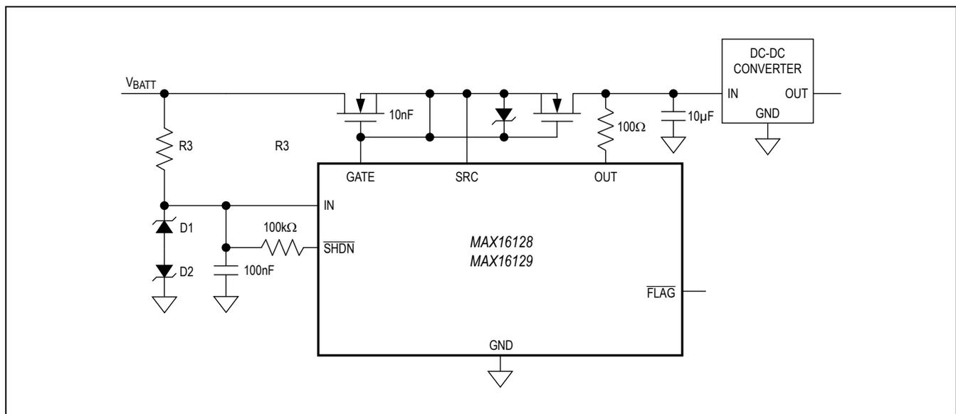
Figure 1. Circuit to Increase Input-Voltage Protection Range
