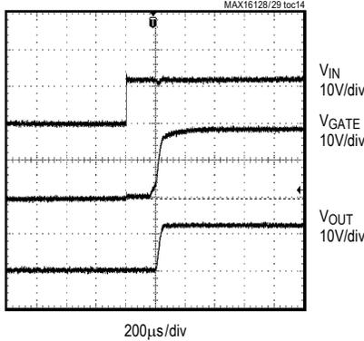
**STARTUP FROM SHUTDOWN ( $\overline{SHDN}$ )**
