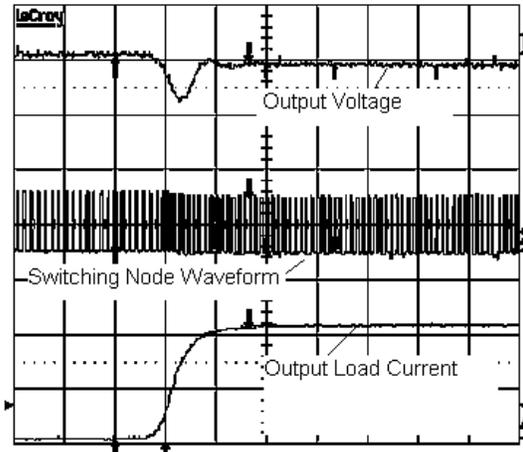
Load Transient Test ( $V_{IN}=5V$ ,  $V_{OUT}=1.2V$ ,  $I_{OUT}= 4A$  to  $0A$ , Forced Continuous Conduction Mode,  $L_{OUT}=1.3\mu H$ ,  $C_{OUT}=3x22\mu F$ , Channel 1: 50mV/Div, Channel 2: 5V/Div, Channel 4: 2A/Div, Time: 10µs/Div)
