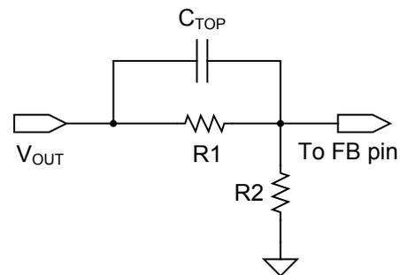
**Figure 8 — Capacitor Coupling to FB Pin**
