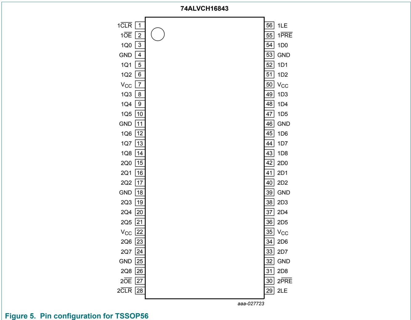
Figure 5. Pin configuration for TSSOP56
