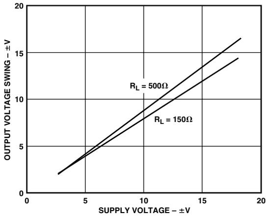
TPC 2. Output Voltage Swing vs. Supply Voltage
