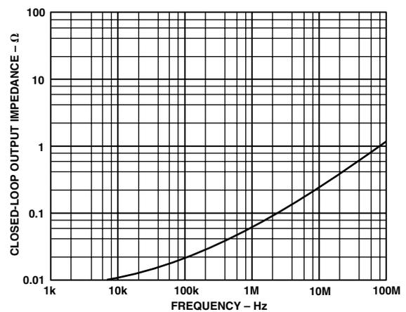
TPC 6. Closed-Loop Output Impedance vs. Frequency
