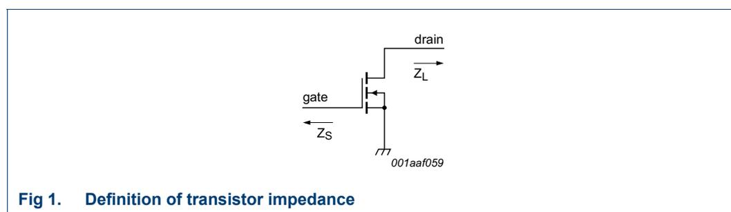
**Fig 1. Definition of transistor impedance**
