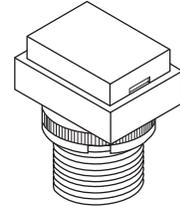
The bezel is an integral part of the switch body. One mounting nut AT057 supplied with each switch.
