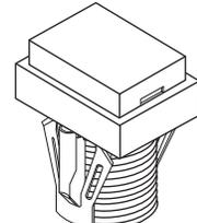
The bezel is an integral part of the switch body.
