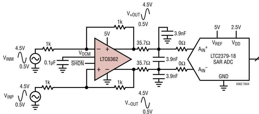
Single-Ended-to-Differential Conversion of a  $4V_{P-P}$  Input with Gain of  $A_V = 2$  to Drive an ADC for Applications Where the Importance of High Input Impedance Justifies Some Degradation in Distortion, Noise, and DC Accuracy. Input Is True High Impedance, However Common Mode Noise and Offset Are Present on the Output. Additionally, When the Input Signal Exceeds  $2.8V_{P-P}$ , a Step in Input Offset Will Occur That Will Degrade Distortion Performance
