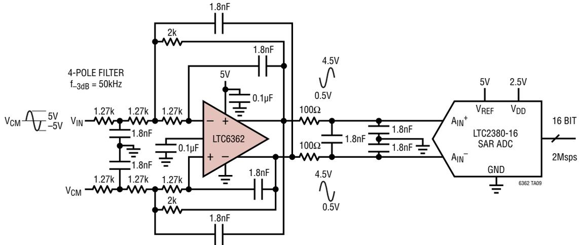
Differential A<sub>v</sub> = 1 Configuration Using an LT<sup>®</sup>5400 Quad-Matched Resistor Network
