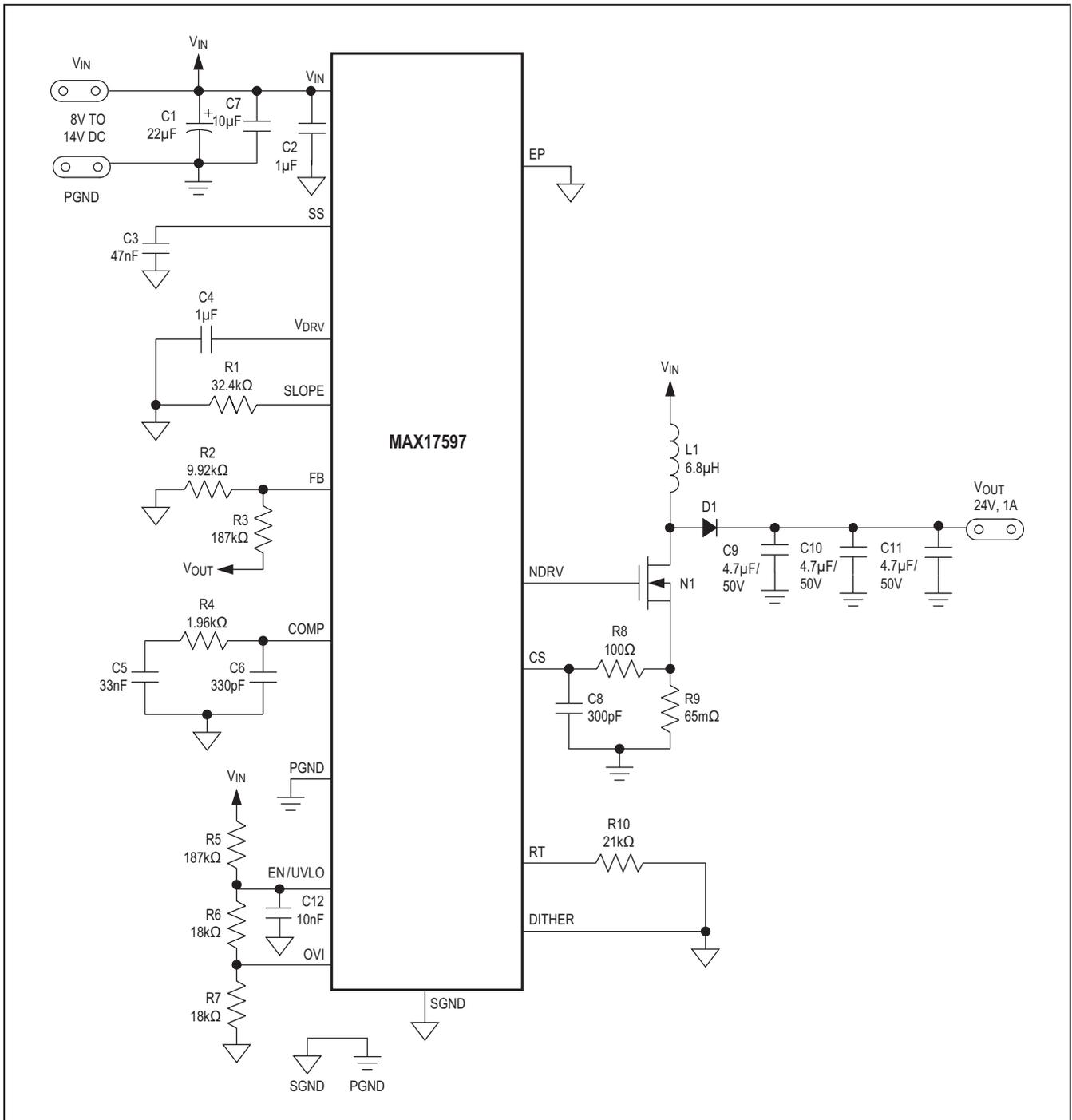
Figure 11. MAX17597 Typical Application Circuit (Nonsynchronous Boost Converter)
