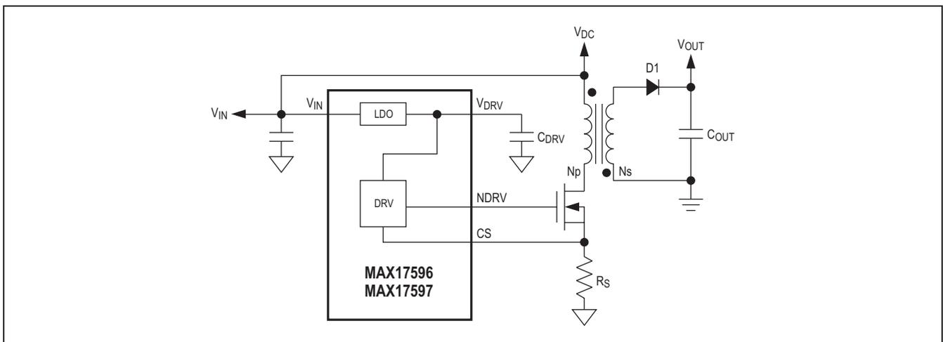
Figure 5. MAX17596/MAX17597 Typical Startup Circuit with V<sub>IN</sub> Connected Directly to DC Input
