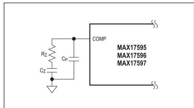
Figure 8. Error-Amplifier Compensation Network
