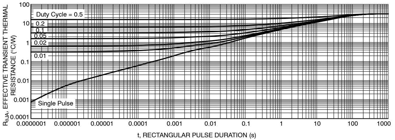
Figure 13. Thermal Characteristics
