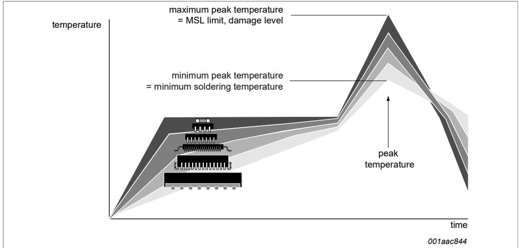
Figure 29. Temperature profiles for large and small components
