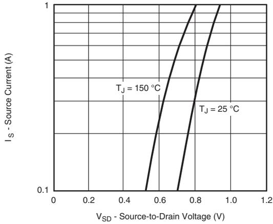
**Surge-Drain Diode Forward Voltage**
