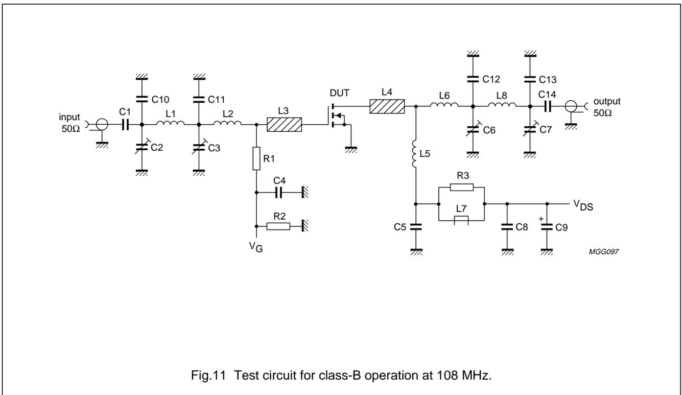
Fig.11 Test circuit for class-B operation at 108 MHz.
