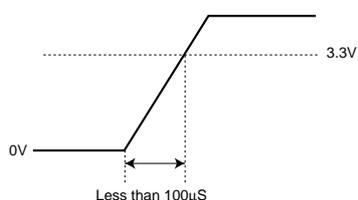
\*3 When the HIGH signal is applied to the CTL pin, a current flows into the CTL pin for a short period until the output rises. Little current flows thereafter.
