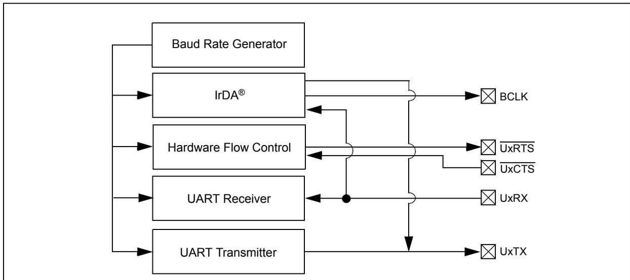
**Note 1:** Both UART1 and UART2 can trigger a DMA data transfer. If U1TX, U1RX, U2TX or U2RX is selected as a DMA IRQ source, a DMA transfer occurs when the U1TXIF, U1RXIF, U2TXIF or U2RXIF bit gets set as a result of a UART1 or UART2 transmission or reception.
