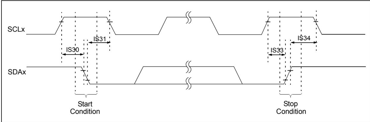
**FIGURE 26-21: I2Cx BUS DATA TIMING CHARACTERISTICS (SLAVE MODE)**
