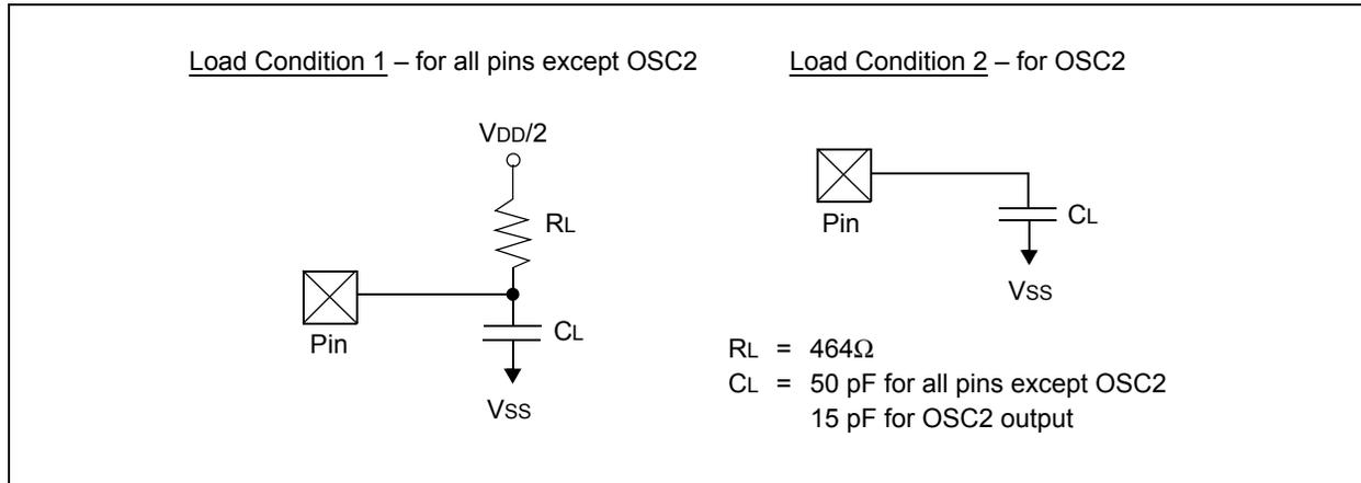
**TABLE 26-15: CAPACITIVE LOADING REQUIREMENTS ON OUTPUT PINS**
