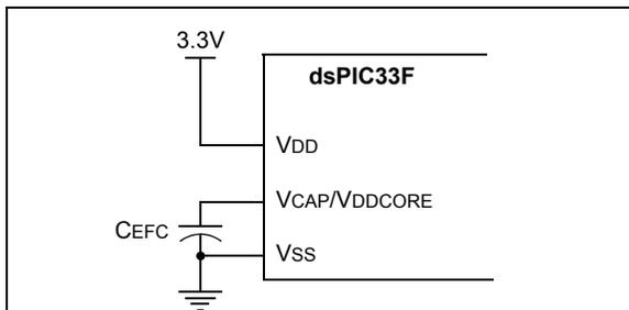
**Note 1:** These are typical operating voltages. Refer to **TABLE 26-13: “Internal Voltage Regulator Specifications”** located in **Section 26.1 “DC Characteristics”** for the full operating ranges of VDD and VCAP/VDDCORE.
