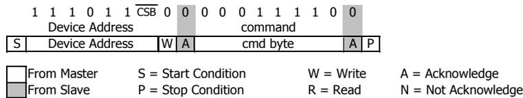
Figure 3: I<sup>2</sup>C Reset Command
