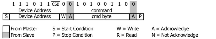
Figure 7: I<sup>2</sup>C Command to read memory address= 011 (Coefficient 3)
