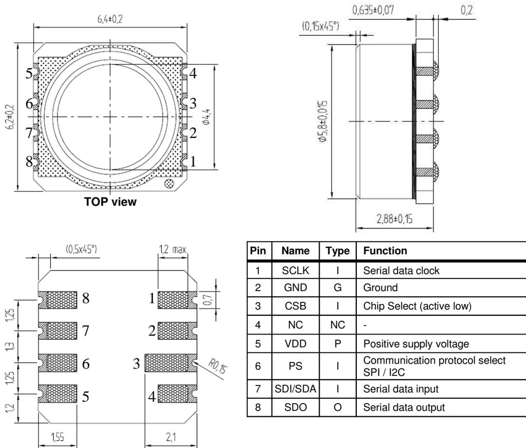
Figure 18: MS5803-30BA package outlines, pin configuration and description
