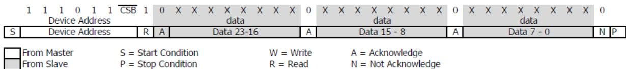
Figure 6: I<sup>2</sup>C pressure response (D1) on 24 bit from MS5803-30BA
