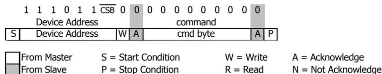
Figure 5: I<sup>2</sup>C ADC read sequence
