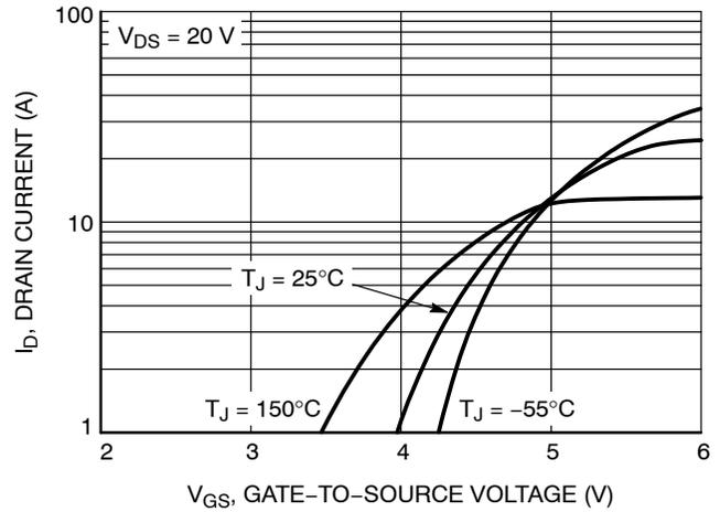
Figure 2. Transfer Characteristics
