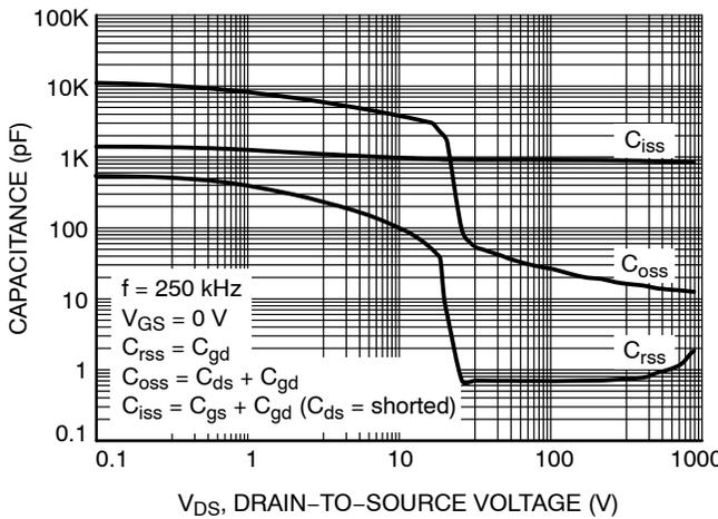
Figure 5. Capacitance Characteristics
