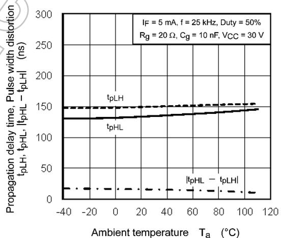
**Fig. 12.2.12  $t_{pLH}, t_{pHL}, |t_{pHL} - t_{pLH}| - T_a$**
