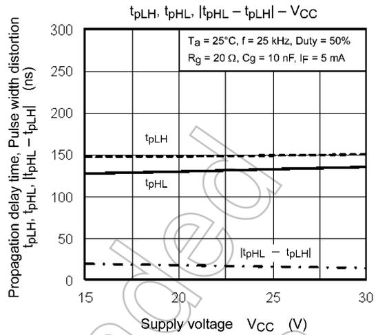
**Fig. 12.2.14**  $t_{pLH}, t_{pHL}, |t_{pHL} - t_{pLH}| - V_{CC}$
