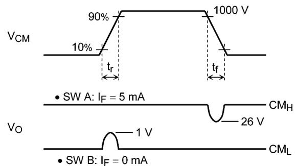
$$CM_H = -\frac{800 \text{ V}}{t_f (\mu\text{s})} \quad CM_L = \frac{800 \text{ V}}{t_r (\mu\text{s})}$$
