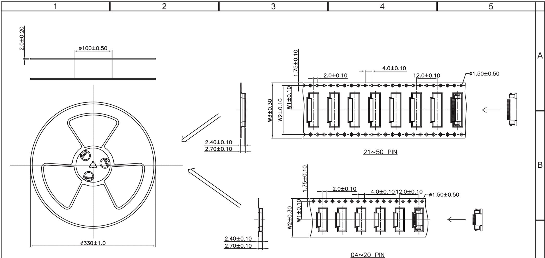
NOTE: 1. 04~06PIN: DIM W1:7.5mm W2:16.0mm PH:12mm
