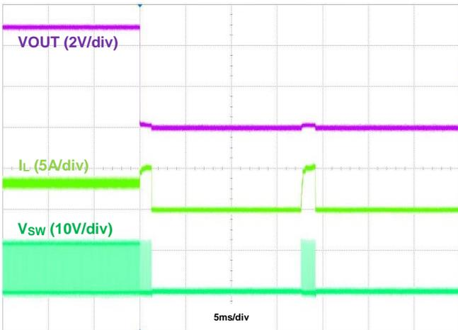
Figure 21. Output Short Protection,  $I_{OUT} = 3.5\text{A}$
