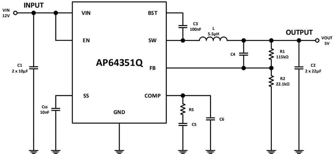
**Figure 27. Example Circuit for Loop Compensation Calculations**
