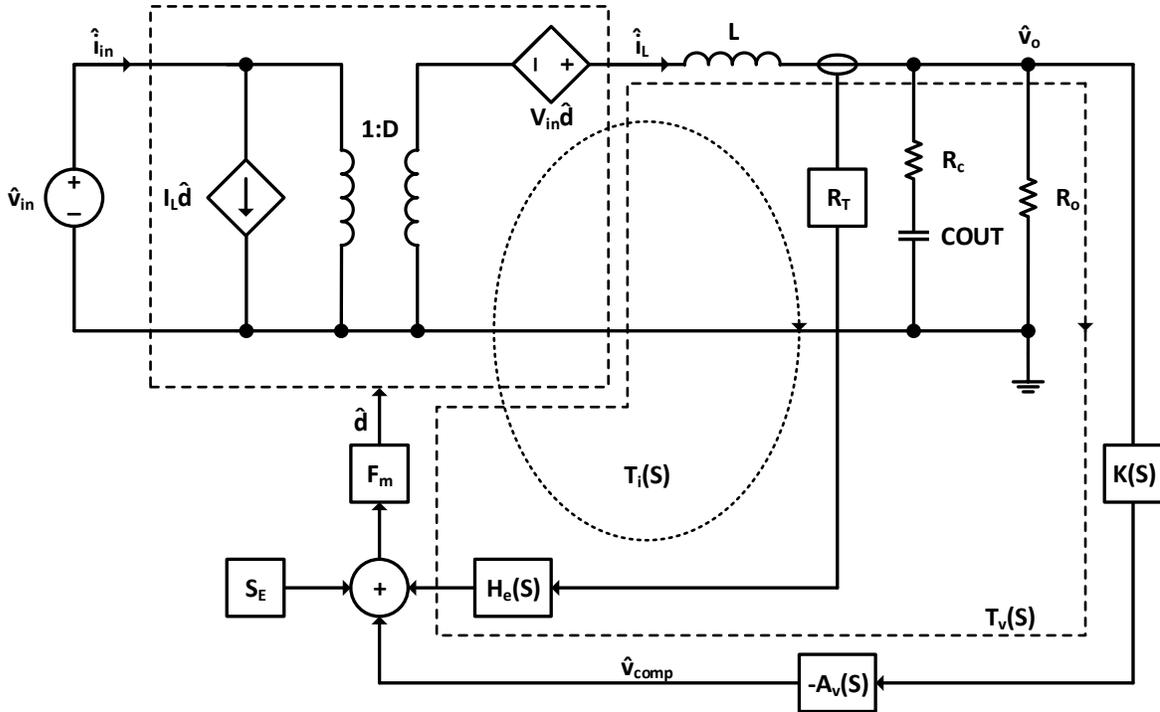
Figure 25. Small Signal Model of Buck Regulator
