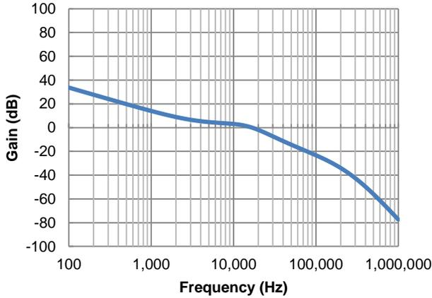
Figure 29. Closed-Loop Bandwidth
