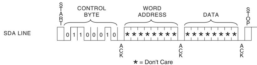
**Figure 9.** Clearing Reversible Write Protect Register (RSWP)
