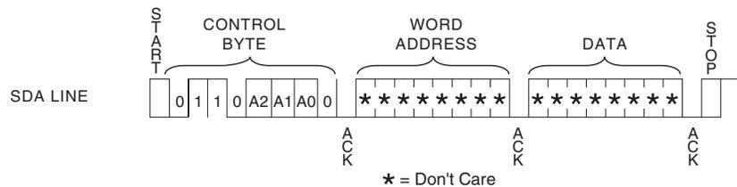
**Figure 8.** Setting Reversible Write Protect Register (RSWP)
