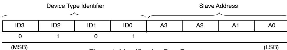
Figure 8. Identification Byte Format
