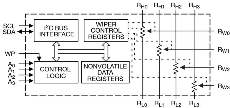
Figure 1. Functional Diagram
