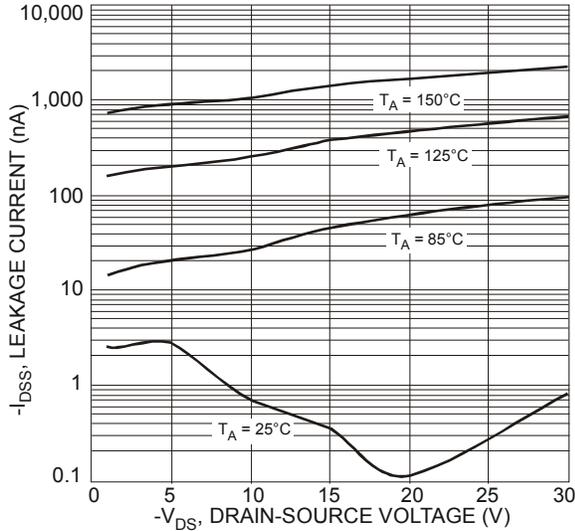
Fig. 21 Typical Drain-Source Leakage Current vs. Voltage
