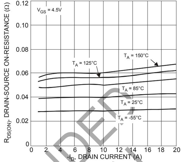
Fig. 16 Typical On-Resistance vs. Drain Current and Temperature
