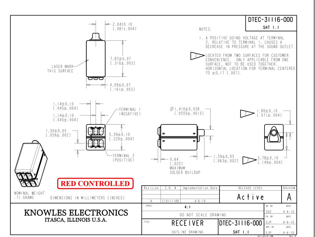
THE DTEC-31116-000 IS A PAIR OF BALANCED ARMATURE RECEIVERS INTENDED FOR USE IN BTE HEARING AIDS. IT HAS A LOW DCR TO IMPEDANCE RATIO, HAS THE CENTER TERMINAL CONNECTED TO CASE AND IS THE SAME SIZE AS AN EF RECEIVER
